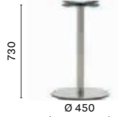
COLUMN Ø 50 TOP MAX 650x650; Ø 900
