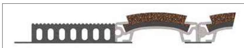
Rubber fill in profiles ensure a neat matwell finish and facilitate cutting on site
